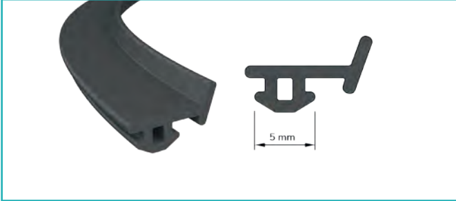
Çakma Conta Nailing Joint
